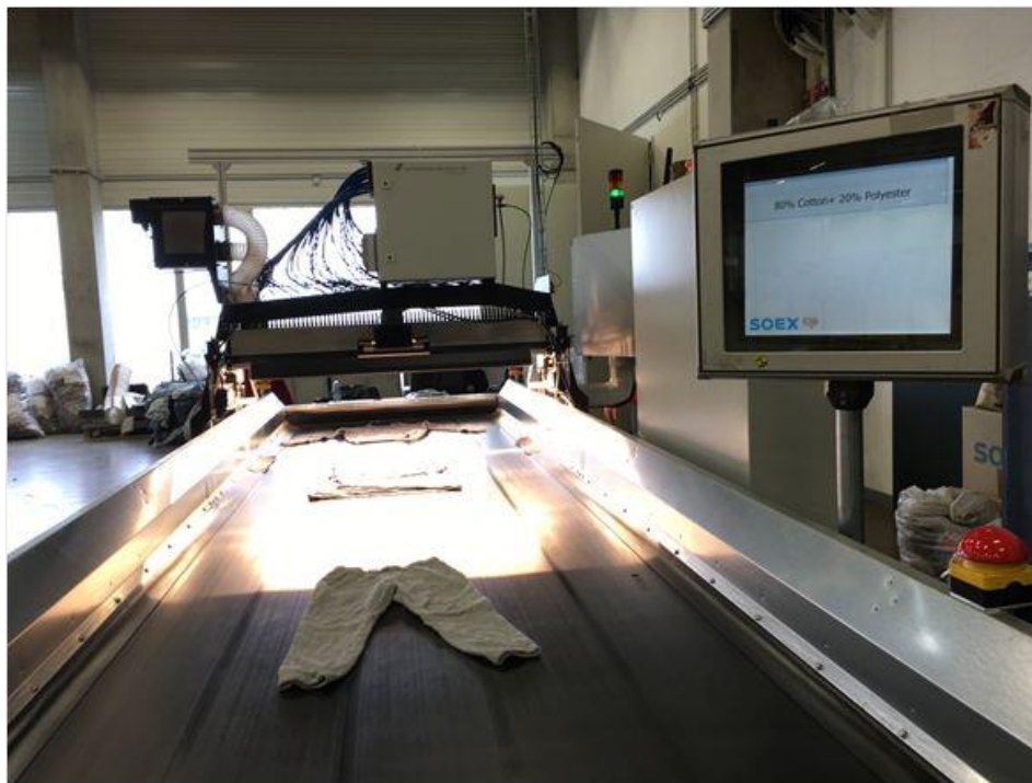
Figure A.2: End of the NIR-sorting line with display of the identified material type.
