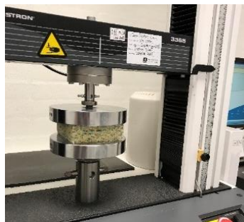
Compression load deflection testing
