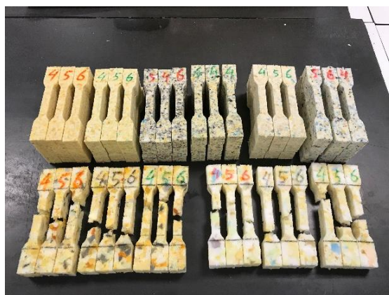
Samples before and after testing of tensile strength
