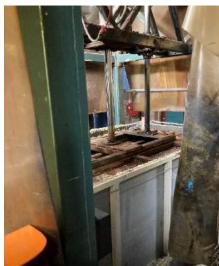
Pressing of the bonded foam block
