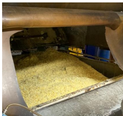
Foam granulates in the mold
