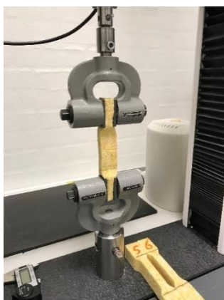
Testing of tensile strength
