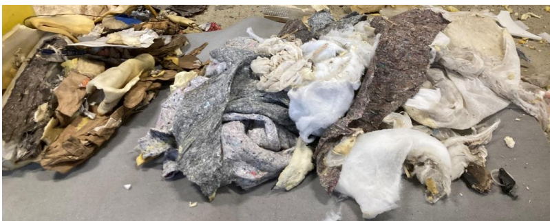
The postconsumer mattress foam from DK contained non-PU-materials including metal parts
